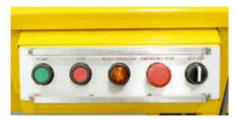
The control panel is conveniently located at the front of the machine therefore alleviating any risk that can be caused by having to lean over to control the machine which can lead to articles of clothing being caught by moving parts leading to possible injury.
