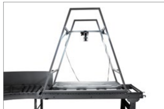
Roller racking camera frame fixed
