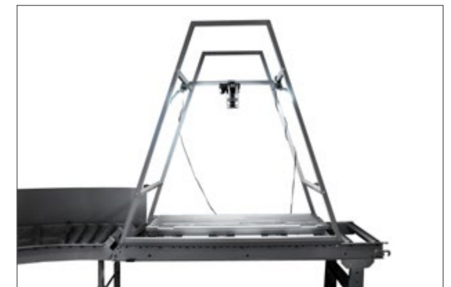
Roller racking camera frame fixed
