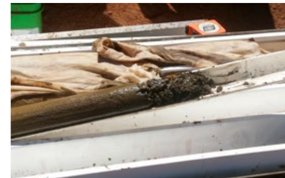
PVC split being used to transfer wet core sample into plastic core tray
