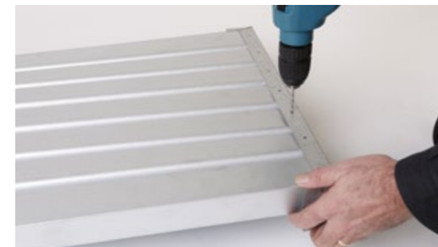
2. Drill rivet holes
